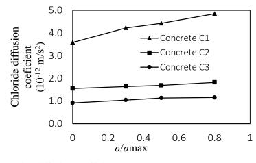
Fig 1 - Increased chloride diffusion coefficient according to the pre-compressive stress in concretes
